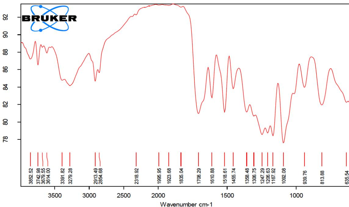
**Figure 4: FTIR spectra of Formulation blend****4.1.4 Solubility of Quercetin (QT) in selected excipients**
