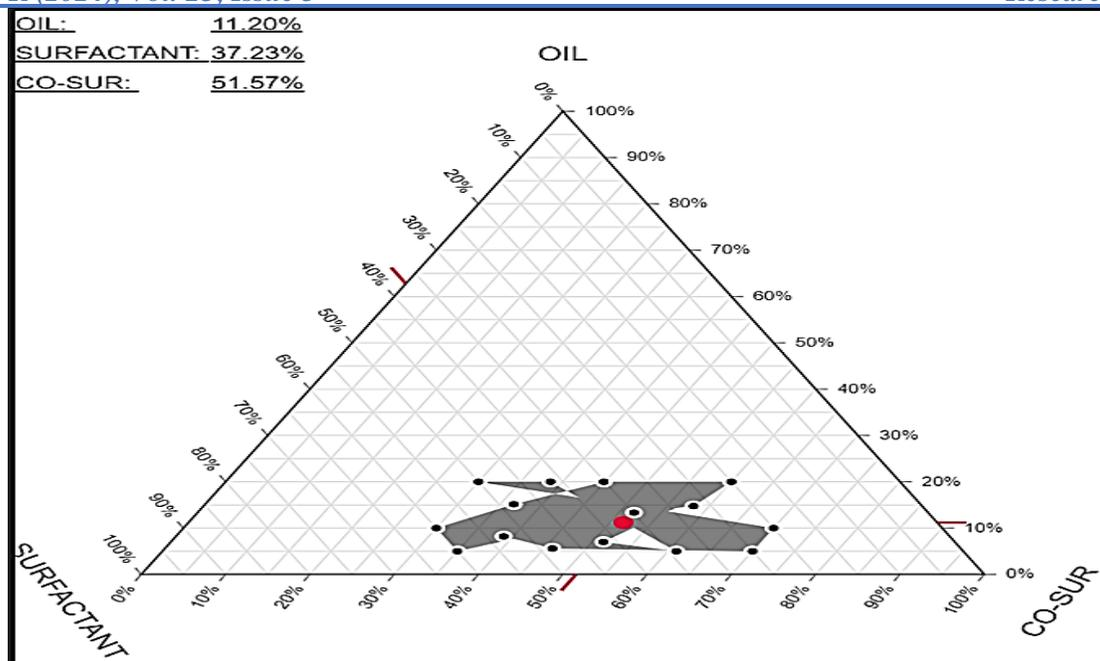
**Figure 6: Pseudo ternary phase diagram of Quercetin (drug), Transcutol P (Oil), Tween 80 (Surfactant) and Propylene glycol (Co-surfactant)**
