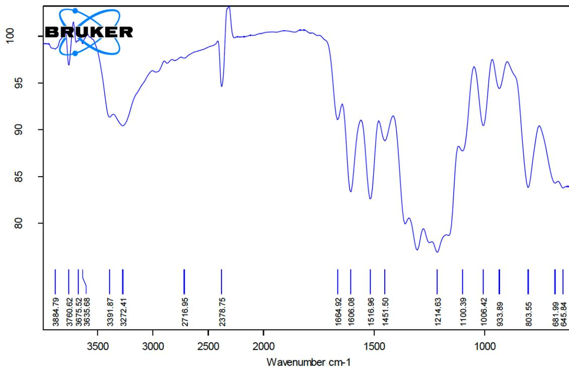
Figure 3: FTIR spectra of Quercetin (Pure drug)
